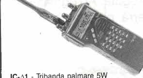
IC-Δ1 - Tribanda palmare 5W VHF 140-470 MHz UHF 400-450 MHz.
